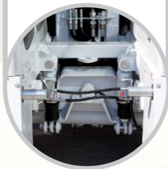
OPTION: CUTTER SUPPORT WITH HYDRAULIC CYLINDERS OR NITROGEN STORAGE CELL
