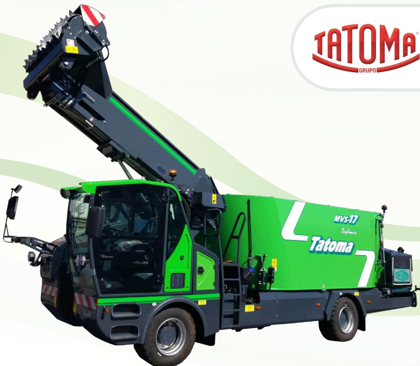
MÉLANGEUSE AUTOMOTRICE VERTICALE DOUBLE VIS
