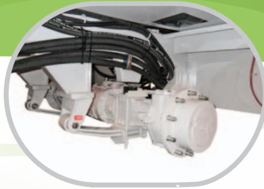
The mixer is fitted with leaf spring front and rear suspension as standard, ensuring maximum operator comfort on rough terrain.
