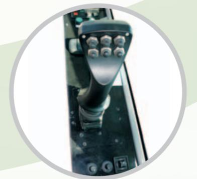
A multi-function joystick is used to provide most of the control operations of the mixer providing accurate, agile handling of the machine.
